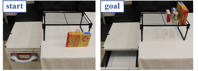
Fig. 7. Kitchen Arrangement Benchmark: Move the objects to the goal positions. The starting position of one of the objects is inside the drawer. In this case, there is both occlusion and uncertainty in execution outcomes.
