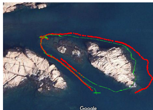
Figure 28: Vehicle's trajectory (green) calculated by its dead-reckoning system and the camera's trajectory (red) estimated by the image-based reconstruction. Both trajectories are shown overlapped with a satellite image of the test scenario (Map data ©2017 Google).
