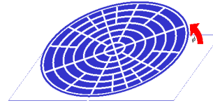
Figure 9: Conceptual design of an actuator array that implements a combined radial-gravity field. Individual actuators are tiled in a circular array pattern. The array is tilted between \phi = 0^\circ and 45^\circ to add a gravity component \delta \mathbf{g} with \delta = \tan \phi .
